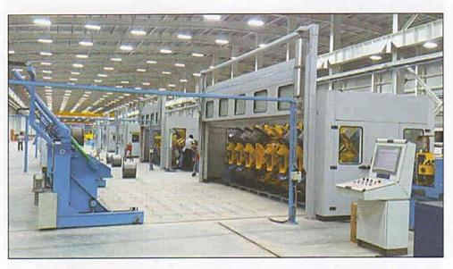
ne of the leading manufacturers of customised rotating machines for stranding, screening and armouring of cables and conductors, Associated Engineers & Industrials Limited (AEI) specialises in reliable, productive and advancedtechnology Rigid Stranding Machines suitable for the production of superior quality stranded conductor for low, medium and extra high voltage (EHV) power cables.
